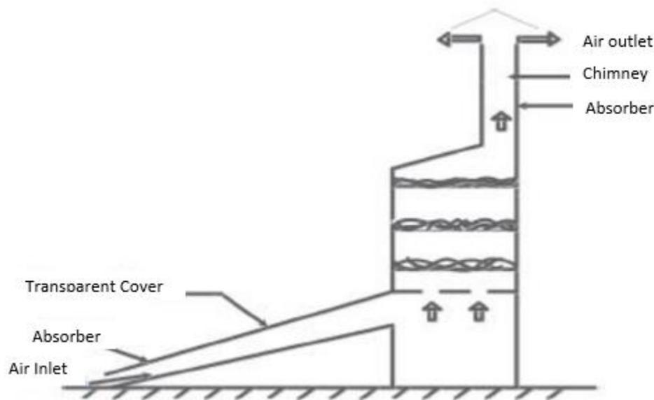
**Figure 2: Illustrates the schematic diagram of indirect solar heater.**
