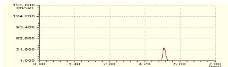
Figure 17: Precision Chromatogram of Standard Pirfenidone at 20  $\mu\text{g/ml}$
