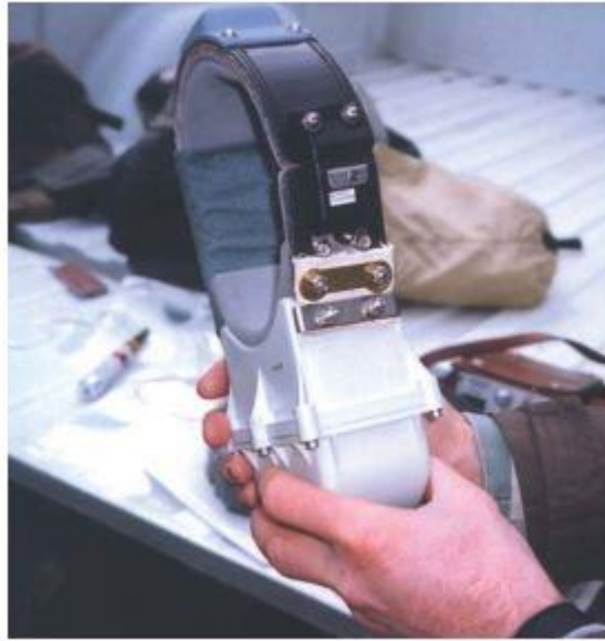
Figure 2: The above figure shows the Radio collar with global positioning system (GPS) technology.
