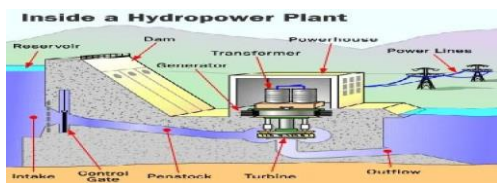
Fig.8: Hydropower Plant Parts
