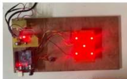
Figure 16: For the number 5 of the dice: lights up the groups 1, 2, 4, 6, 7
