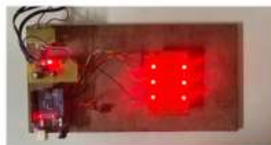
Figure 11: For the number 6 of the dice: lights up the groups 1, 2, 3, 5, 6, 7
