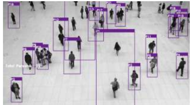
Fig. 10. Tracking of Human using YOLOv8 and Deep Sort
