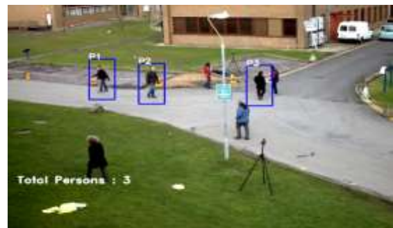
Fig. 3. Tracking in Real Time using CCTVs using YOLOv8
