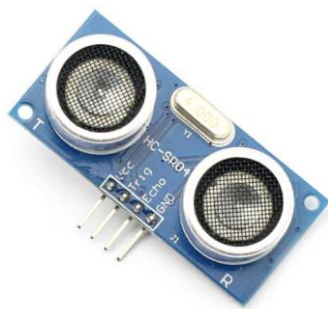
Figure: Ultrasonic sensors
