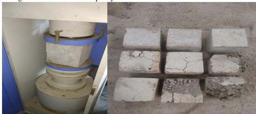
Fig 4.6 compressive testing machine and cubes after test
