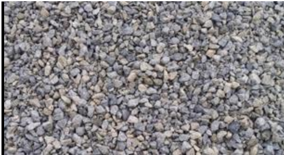
Figure 5: The image of a Coarse Aggregate. The coarse aggregate was sourced locally [civilclick].
