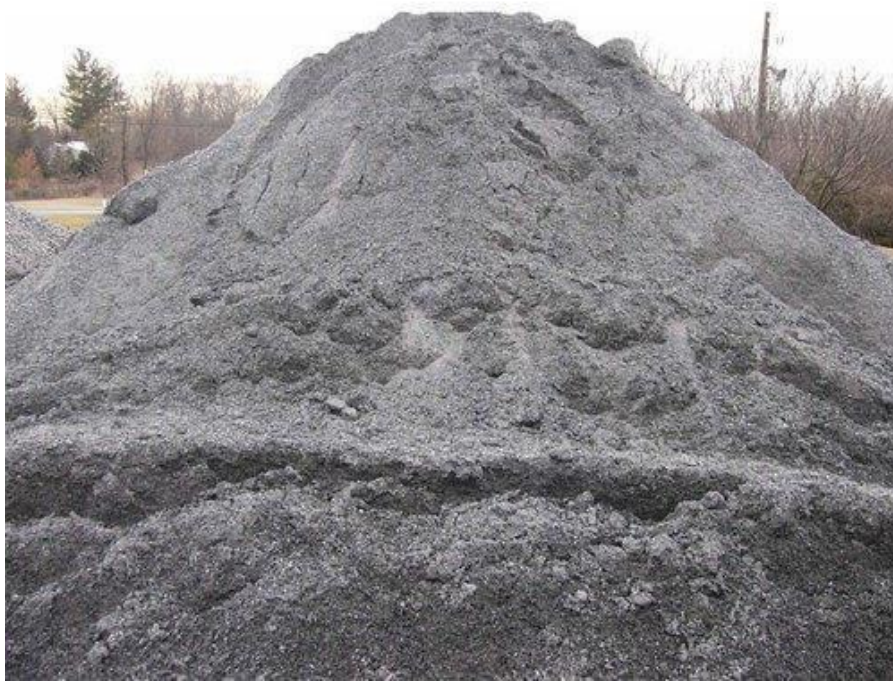
Figure 4: The image of M Sand. M-Sand is a replacement of river sand for the construction of concrete building [Indiamart].
