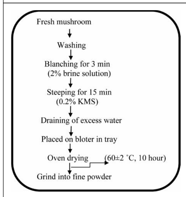
Figure 1: Flow Diagram of Processing of Mushroom
