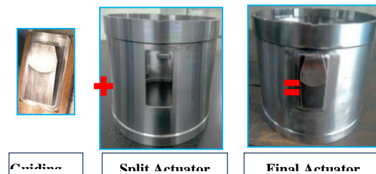
Figure 16 Prototype of Actuator Housing (Split)
