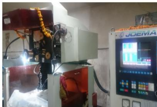
Fig-1: Joe marswtt-655 Taiwan make wire cut machine
