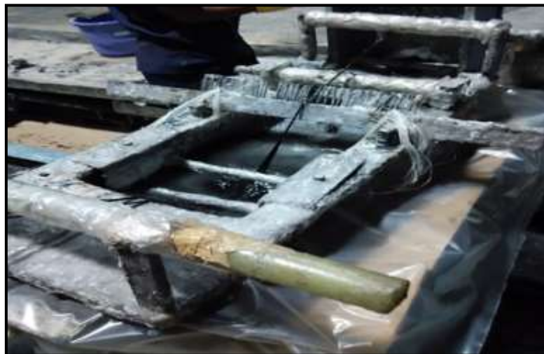
Figure 2.3: Creating fiberglass drive shaft (a)
