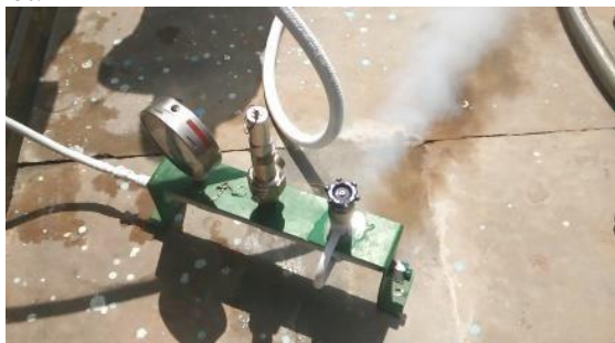
Fig. 4.4 Pressure Gauge – Globe valve setup
