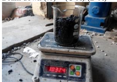
Fig 4.3 Drain down test
