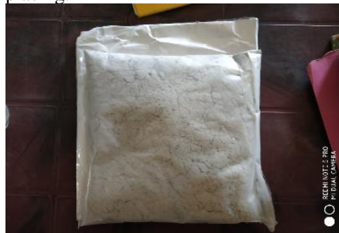
Fig 3.4 Stabilizing Additive (Cellulose Fibers)
