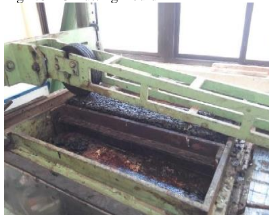
Fig 4.7 Immersion Wheel Tracking Machine for Conducting Rutting Test
