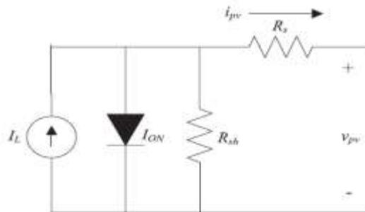
Fig.3.2 Equivalent circuit diagram of the PV cell
