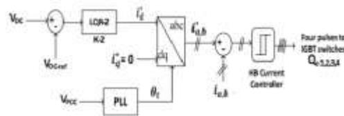
Fig. 6. Control blocks for the GSI.
