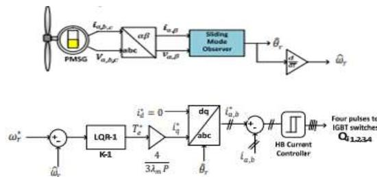
Fig. 5. Control blocks for the MSC.
