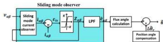
Fig. 3. Schematic diagram of the rotor position estimation using SMO.
