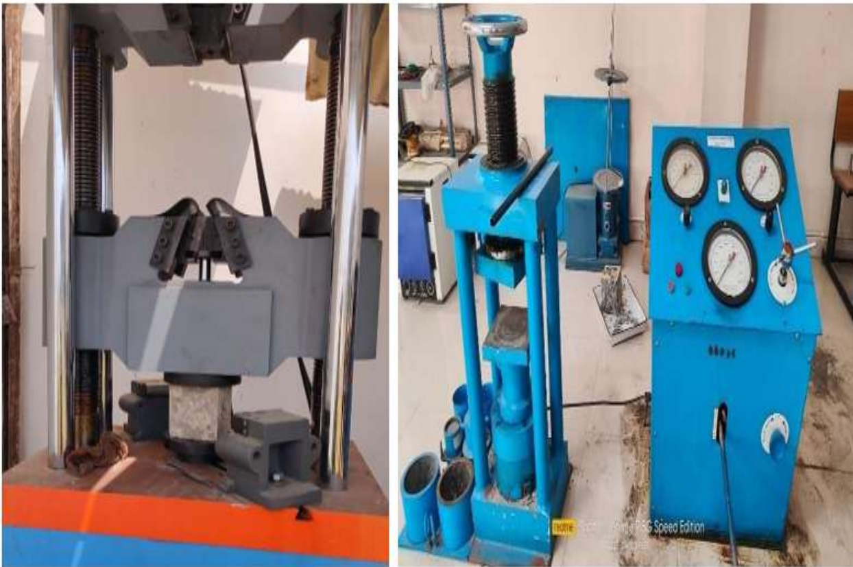
Fig 1: Test set up at REC Azamgarh for compressive strength test of concrete.
