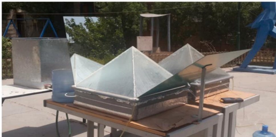
Fig- 3 solar distiller with mirror & cords wick
