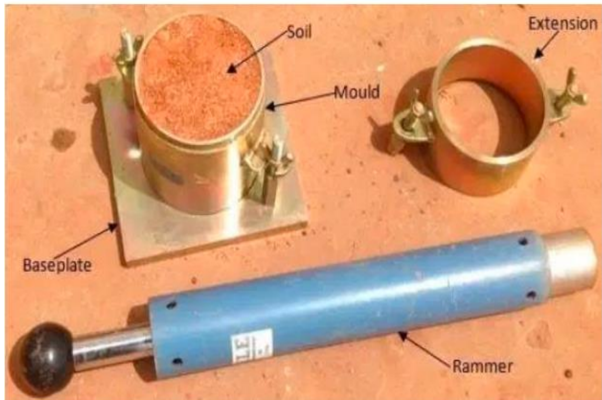
Figure 4 Standard proctor test
