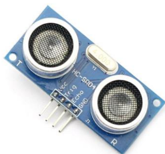
Figure: Ultrasonic sensors
