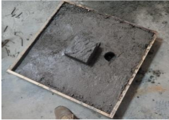
Fig 1: Flat Plate Specimen with & without opening
