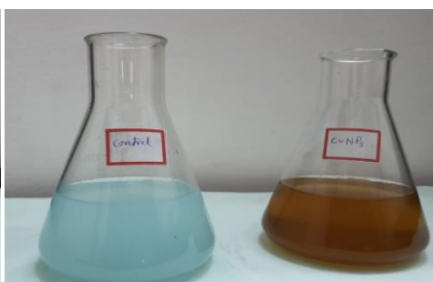
Figure 3.3: Colour change indicating synthesis of CuNPs
