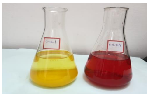
Figure 3.2 : Colour change indicating synthesis of AuNPs
