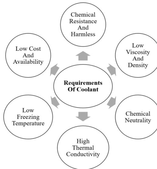
**Figure 1: Illustrates the Basic Requirements for Selecting Any Coolant for Different Machining Processes.**
