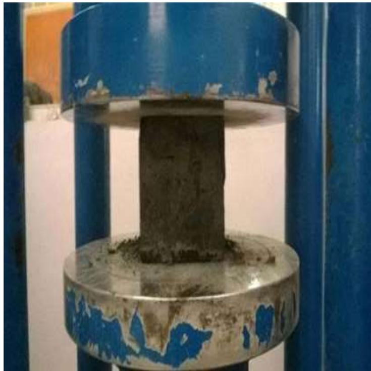
**Figure 7: Compression testing machine**
