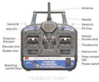
Figure:10 Frequency transmitter
