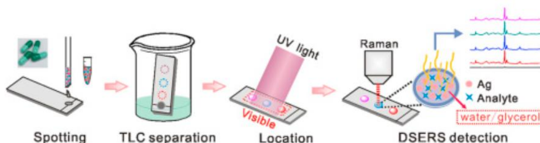
Figure 1: Highly Sensitive On-Site Detection Of Pharmaceuticals Contaminated In Botanical Dietary Supplements Utilizing Thin Layer Chromatography Coupled With Dynamic Surface Enhanced Raman Spectroscopy.
