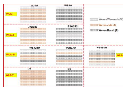
Figure 1: Jute fiber location and layer arrangement of composites
