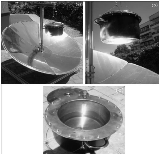
Fig. 2.2: (a) Cooker A in operation. (b) Focused sun on utensil. (c) Inner pot view with water
