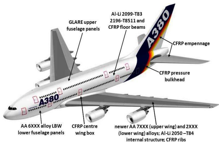
Fig. 2. Different parts of airbus 380 made up with light weight alloys of aluminium [9].
