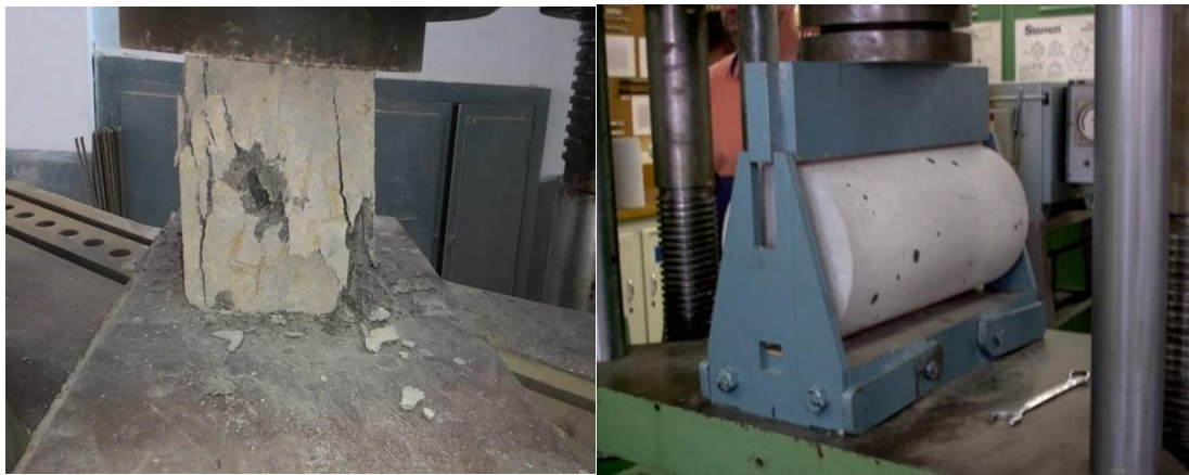
Figure: 4.3 After testing Compression test Split tensile testing
