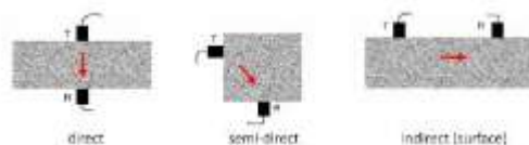
Figure 4.2.1. Ultrasonic Pulse Velocity Test
