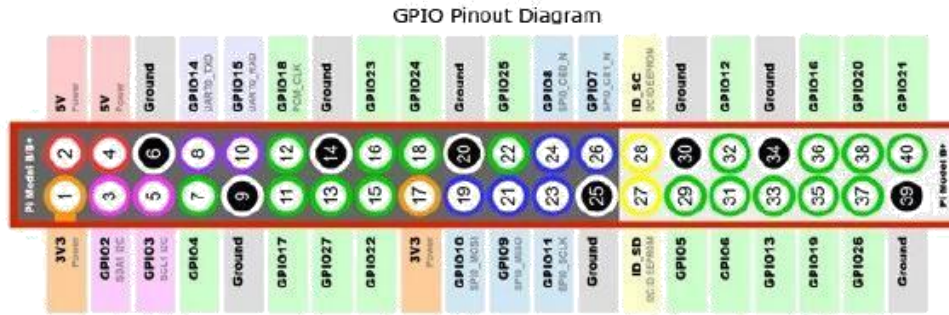
Figure.2 Raspberry pi GPIO pinout diagram
