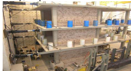
Figure 1 : Test Structure with Infill Walls
