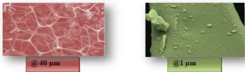
Fig 2: MS, Fe 3 O 4 /MS, and PDMS@Fe 3 O 4 /MS scanning electron micrographs at 1 μm and 40 μm
