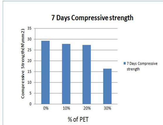
Table 5.2 values for 0% replacement of fine aggregate with polyethylene terephthalate
