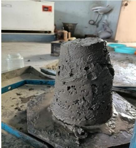
**TABLE 4.2: TEST RESULTS OF SLUMP WITH DIFFERENT %REPLACEMENT OF SAND WITH POLY ETHYLENE TEREPHTHALATE**
