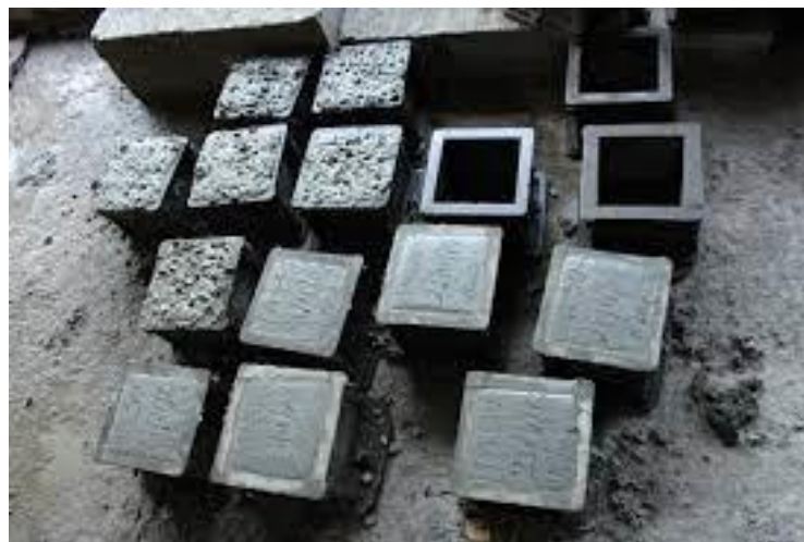
Fig. 13: Compacted concrete cubes.
