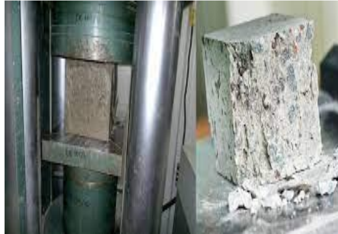
Fig. 15: Compressive strength test on concrete cubes.
