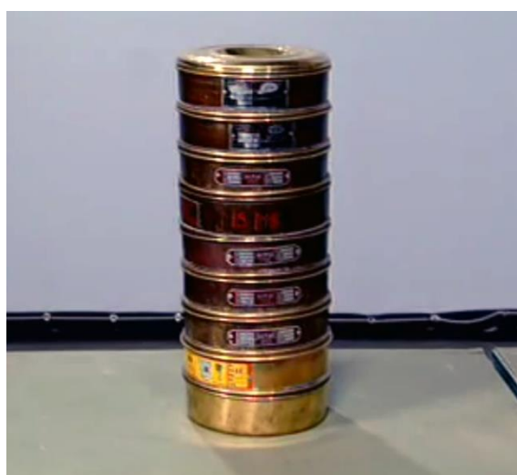
Fig. 1: Sieves for fine aggregates.
