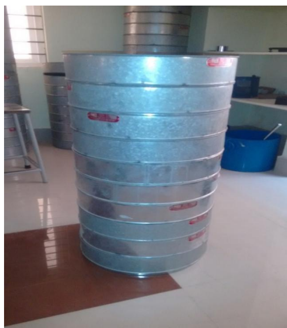
Fig. 2: Sieves for coarse aggregates.
