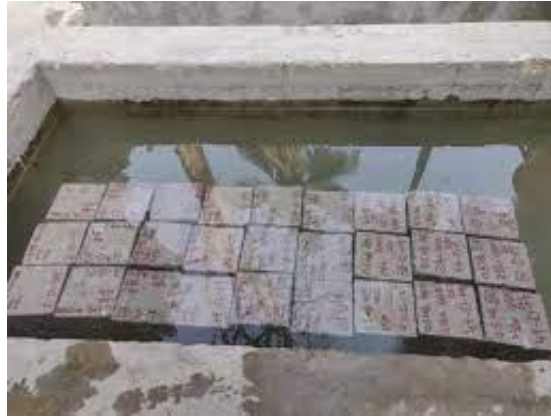
Fig. 14: Water curing of concrete specimen.
