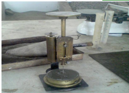
Fig. 6: Initial setting time
