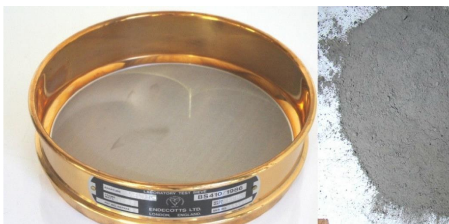
Fig. 7: Cement fineness test.
