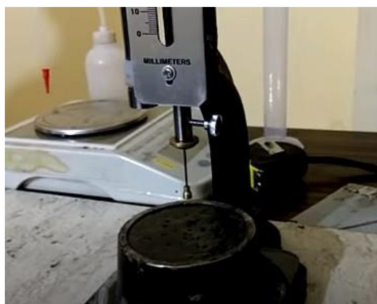
Fig. 5: Final setting time.
