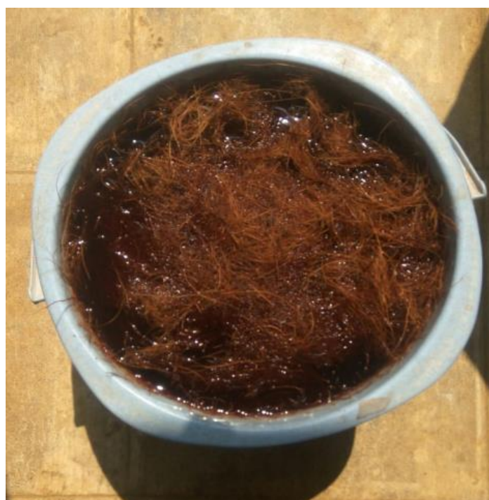
Fig. 11: Oil immersion of coconut fibre.
