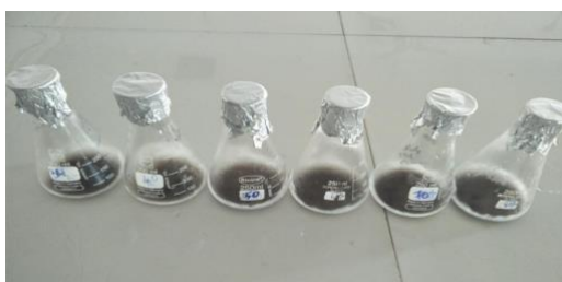
The above picture depicts the saturation of crude extract from 30%-80% and deep freezing at 4°C (Ammonium sulphate precipitation)
