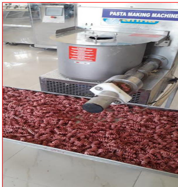
Figure 1: Preparation of pasta using single screw extruder
