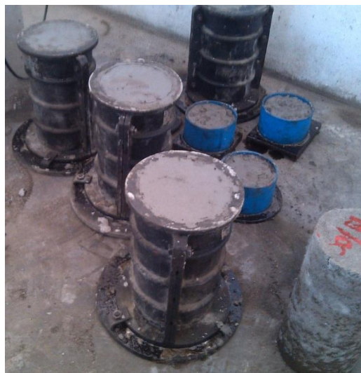
Fig 6.2 casting of specimen
