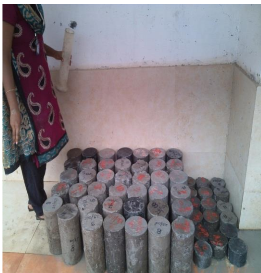
Fig 7.1 Cylinders after Curing Left For Air Drying For 24 hrs.
