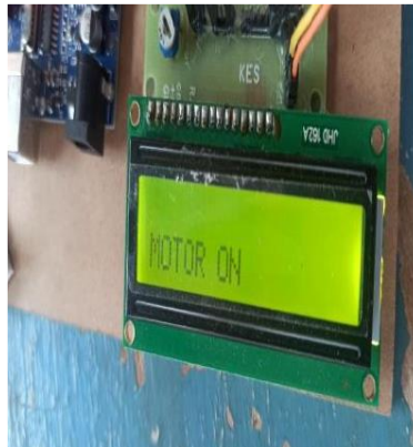
Fig 3: LCD Display the motor is on
