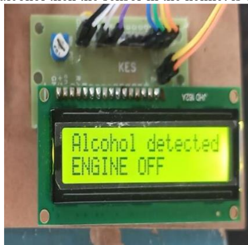
Fig 4: LCD display the alcohol detected warning
