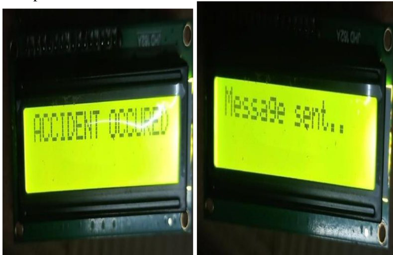
Fig 6: LCD display the accident occurred Fig 7: LCD display the message sent
