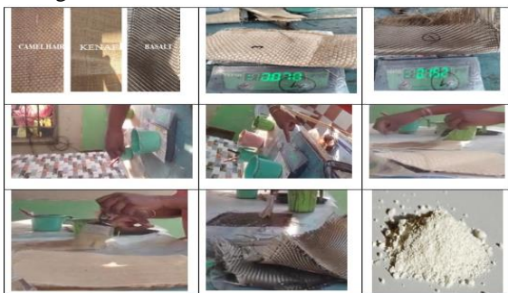
Fig8: COMPLETE SEQUENCE OF PECIMEN MAKING PROCESS
