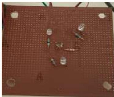
Fig. 2: RGB LED's and Phototransistor arrangements
