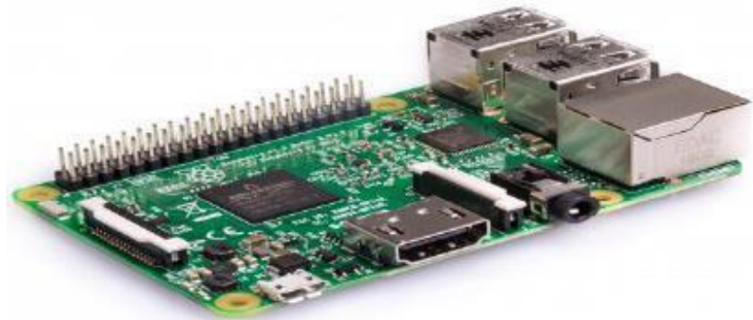
Figure.1 Raspberry pi 3b
