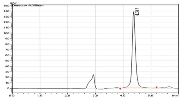
**Fig. 4. HPLC Chromatogram for rutin standard (40 ppm)**
