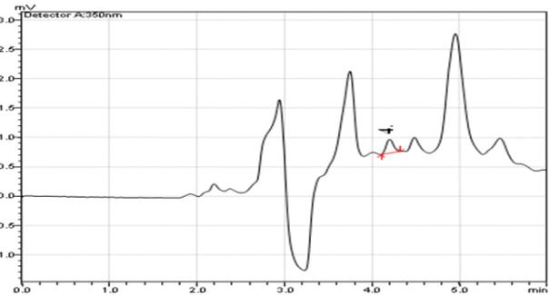
**Fig. 5. HPLC Chromatogram for SC-CO<sub>2</sub> extraction of rutin at 40 °C, 100 bar and 40 min**
