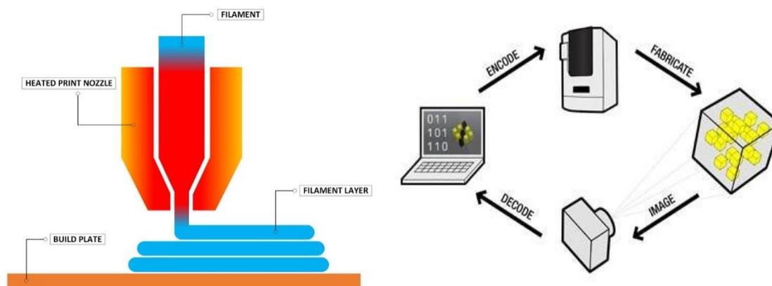
Fig. 1: Working principal of 3D printer [Cao, Marmik]
