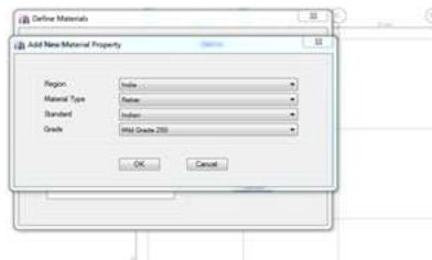
Fig: 4 Defining the mid steel bars for the lateral reinforcement tie bars as per IS codes
