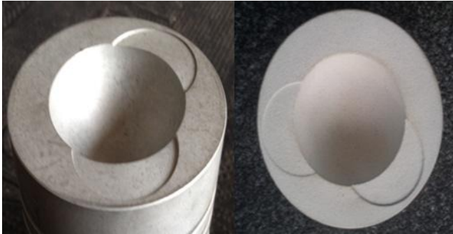
Fig 3. Uncoated baseline engine piston (left) and YSZ coated piston (right).
