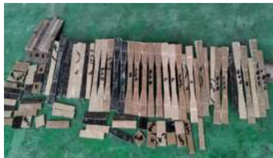
Fig10: All 7 compositions of Tensile, Flexural, Hardness and Impact specimens after cutting into ASTM standards
