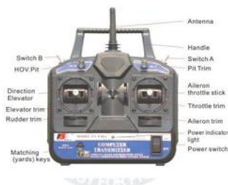
Figure: 10 Frequency transmitter
