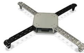
Figure 4 Modeling and rendering of a Quadcopter Drone in fusion 360
