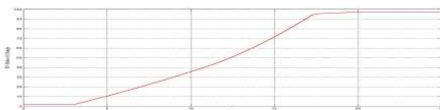
Figure 15: EV Battery Charging Conditions using SVM Controller
